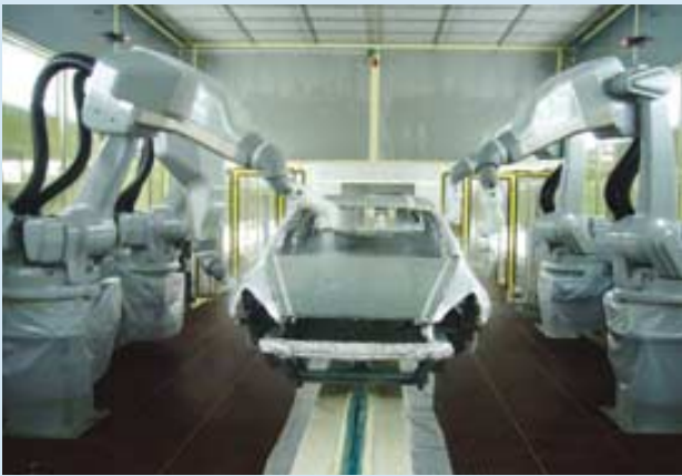
Second Auto Plant at Guangzhou Honda To reduce emissions of volatile organic compounds, water-based paints are used for the middle and top coats of paint. Paint is sprayed on with a special water-based paint gun to improve coating efficiency.
