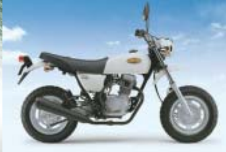
Ape 100: Equipped with a 5-speed transmission and air-cooled 4-stroke OHC single-cylinder engine, the Ape 100 is a sport minibike that delivers the handling and control enjoyment associated with larger motorcycles.
