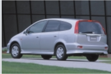
Stream: The new Stream 7-passenger minivan is developed based on the same "Global Compact Platform" used in Civic models. It is powered by the new 2.0-liter DOHC i-VTEC engine or the 1.7-liter SOHC VTEC engine.
